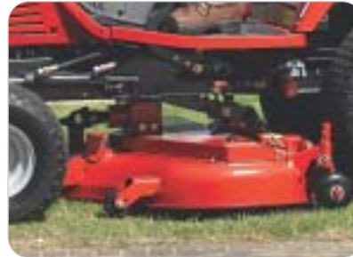
The cutting platform has six height settings and electro-hydraulic lift
