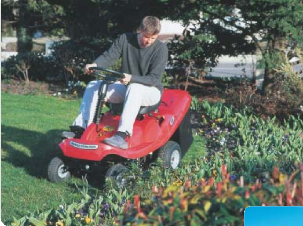
Left: MF 2107. 630 mm cut and 140 litre collection. Small, compact and highly manoeuvrable
