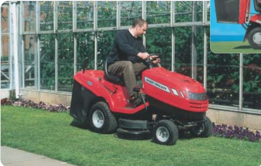
Above: MF 2314. showing the easy-to-empty collector
